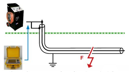
Surge Generator Fault Prelocation Principle
