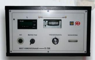
The bridge S-709 was intended for distance and fault locating in power cable lines with the help of bridge methods (of Muller, Kupfmuller, Hilborn/Graf), and distance definition to the place of fault in the power cable shield.
